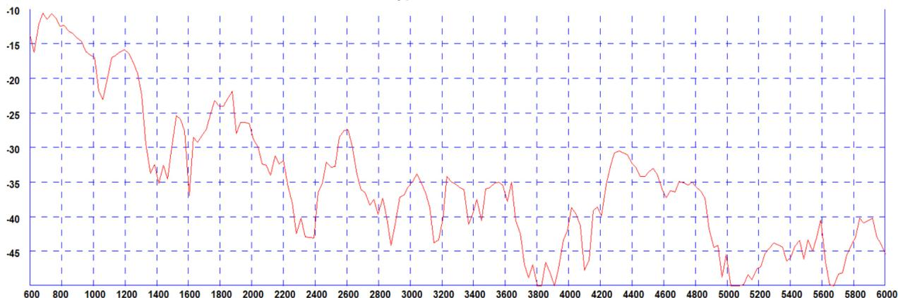
\*\*\*Typical isolation measured on a 600x600mm (2'x2') ground plane without cable loss
