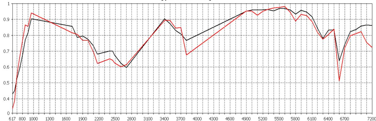
\*\*\*Efficiency simulated in CST Microwave Studio with all elements fed together without cable loss in free space
