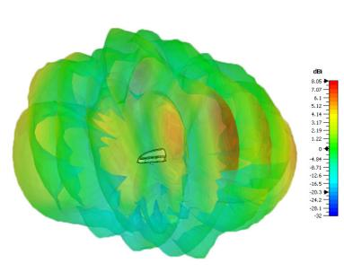
3D patterns all simulated in CST Microwave Studio with all elements of same type fed together excluding cable loss
