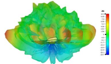
3D patterns all simulated in CST Microwave Studio with all elements of same type fed together excluding cable loss
