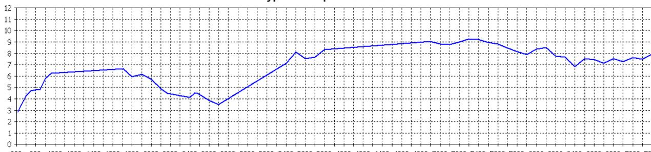
\*\*Swept peak gain simulated in CST Microwave Studio with all elements fed together without cable loss on 600x600mm (2'x2') ground plane
