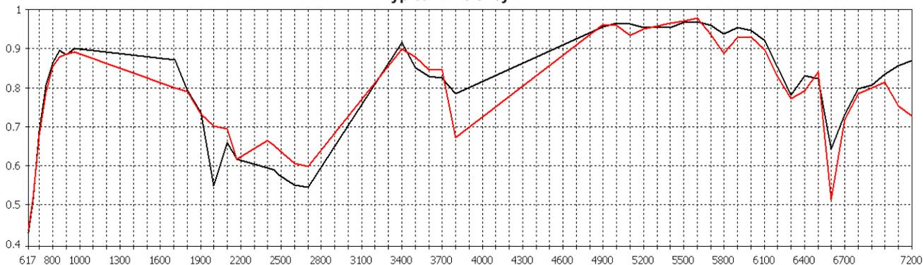
\*\*\*Efficiency simulated in CST Microwave Studio with all elements fed together without cable loss on 600x600mm (2'x2') ground plane
