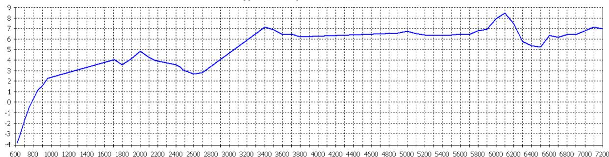
\*\*Swept peak gain simulated in CST Microwave Studio with all elements fed together without cable loss in free space
