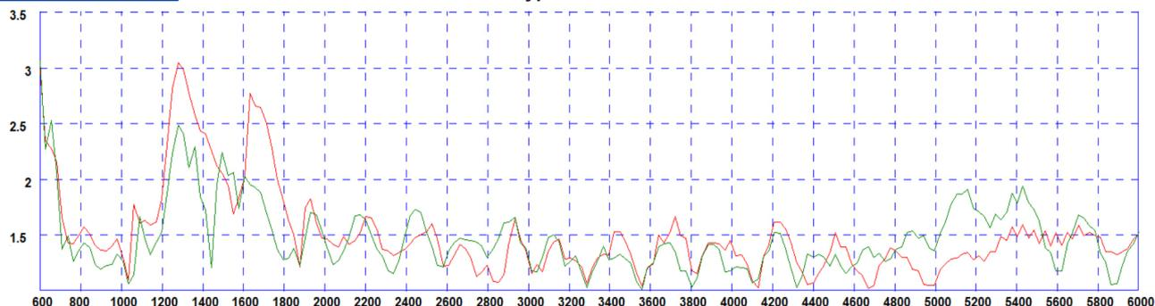
\*VSWR elements 1&2 measured on 600x600mm (2'x2') ground plane without additional cable
